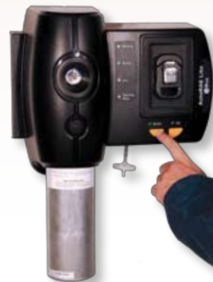
Bump testing ToxiRAE 3 with AutoRAE Lite Bump Test and Calibration Station
